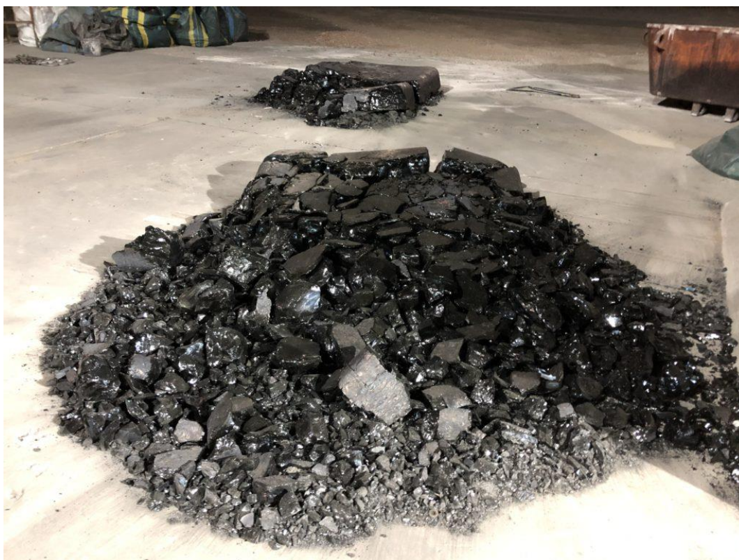
Stabilized arsenical glass using DST’s GlassLock Process Credit: Dundee Sustainable Technologies
